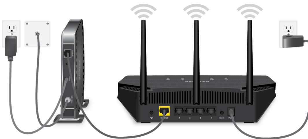
Figure 6. Cable your router
