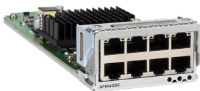
8x10GBASE-T Port Card - 100M/1G/2.5G/5G/10G (APM408C)
