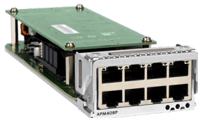
8x10GBASE-T PoE+ Port Card - 100M/1G/2.5G/5G/10G (APM408P)
