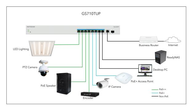
$<sup>\</sup>star$  GS110TUP and GS710TUP can support, but are not limited to, power the devices shown in the above examples.
