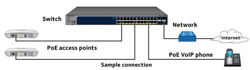
1. Connect devices to the RJ-45 PoE network ports on the switch front panel. Use Category 5e (Cat 5e) Ethernet cables terminated with RJ-45 connectors to make Gigabit connections.
